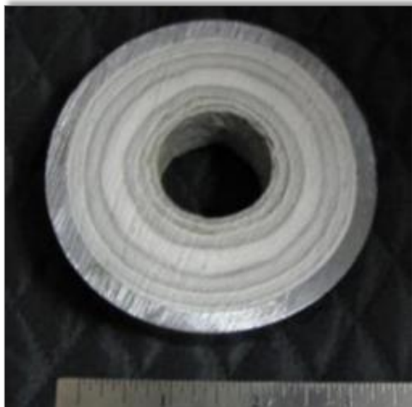
Deposits in 3 inch steam line, result of repeated instances of boiler water carryover
