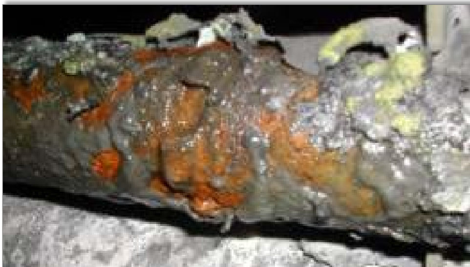
External deposits containing sulfur compounds— from burning high sulfur oil
