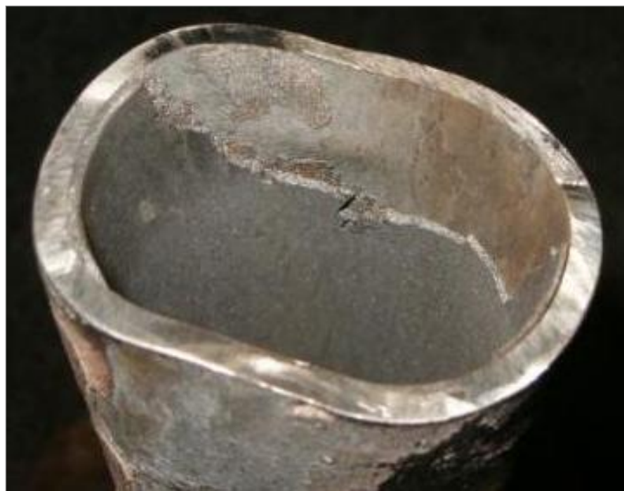
Heavy magnetite formation in a superheater tube
