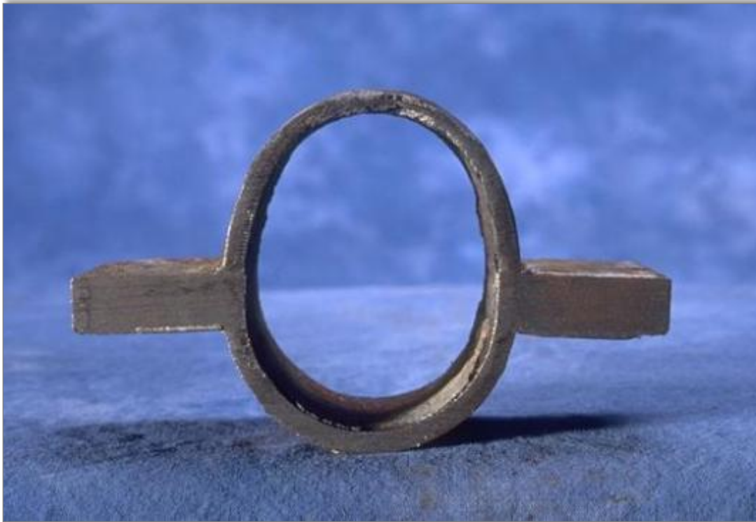
Generating tube elongated due to slow metal creep from long term overheating
