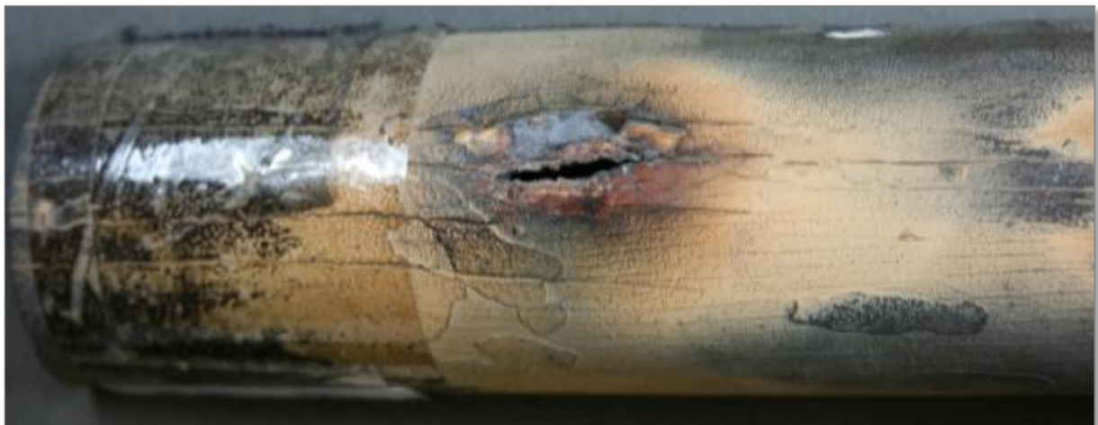
Superheater tube failure promoted by internal surface deposits
