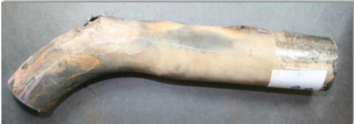
Superheater tube bulges
