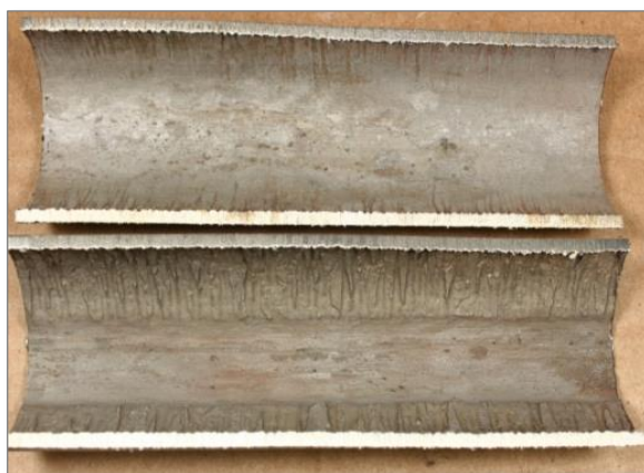
Corrosion and failure on the lower surface of a horizontal line etched due to low pH when steam condensed
