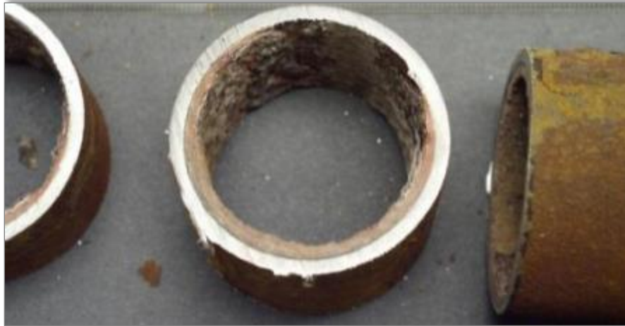
Boiler tube with iron and silica scale
