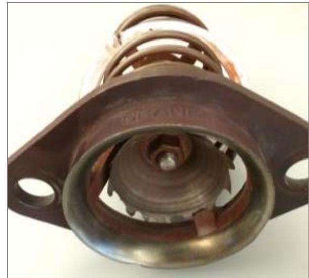
Mechanically damaged deaerator spray valve
