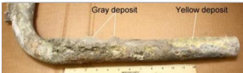
Bare economizer tube sections before cleaning
