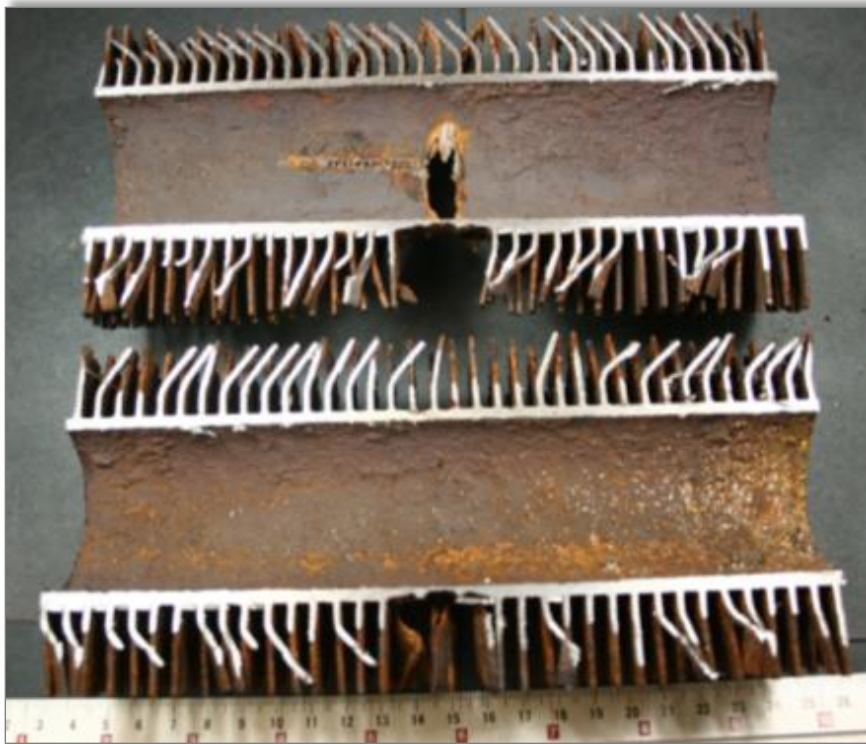
Tube removed and split longitudinally, before cleaning
