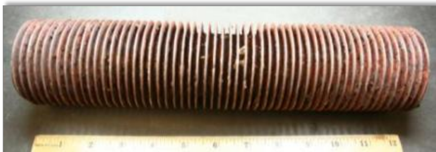
Finned superheater tube removed from a HSRG
