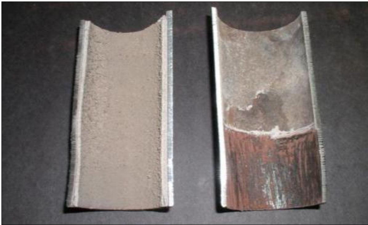
Tube mineral scale removed for deposit weight density determination. Scrape and weigh method vs. glass bead blasting
