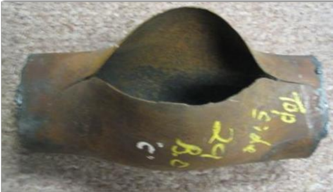
Thin lip failure due to rapid overheating
