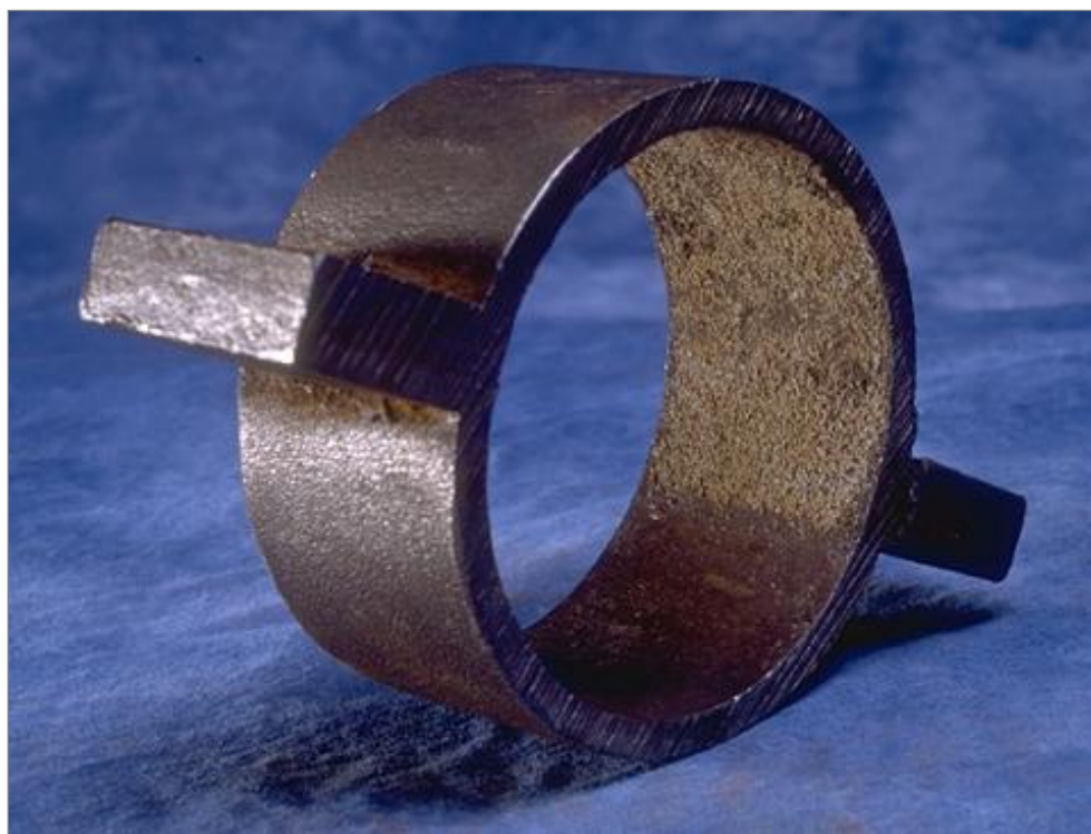
Rare example of a furnace wall tube section showing the effect of differential deposition from furnace zone radiant heat input (top side) vs. convection zone return gas passage (bottom side).
