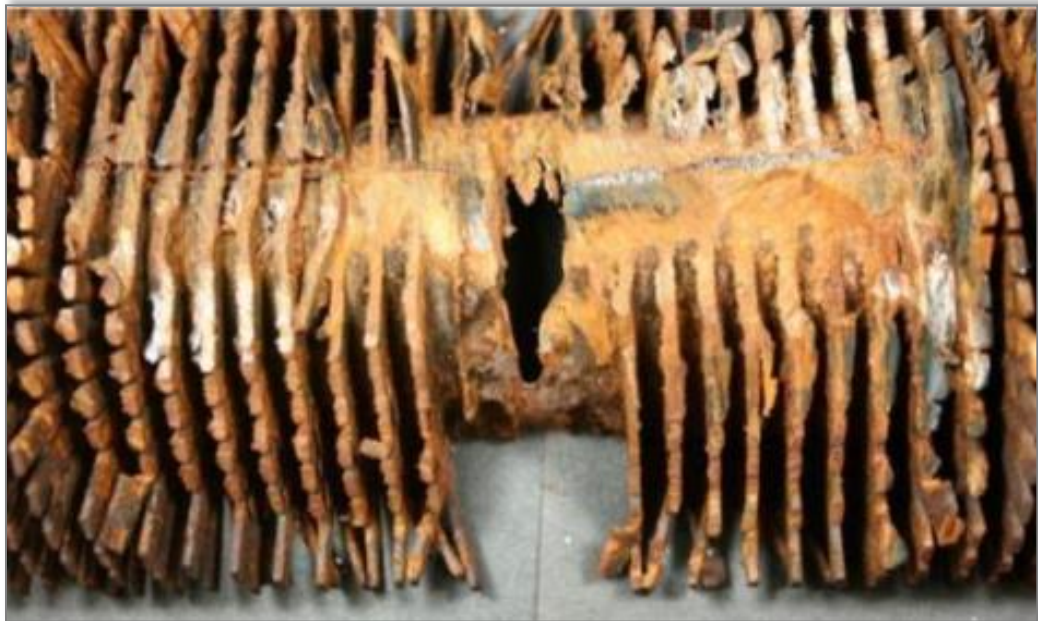
Finned economizer tube failure
