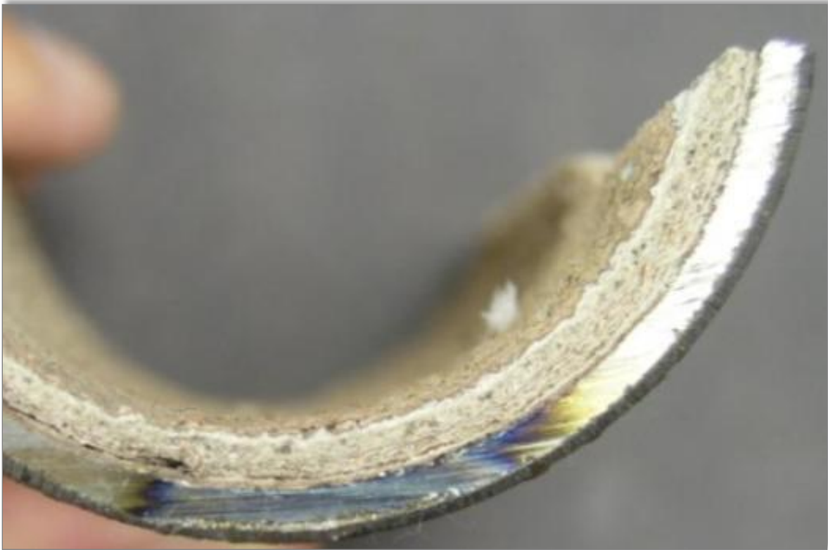
Tube scale layering due to multiple feedwater hardness excursions
