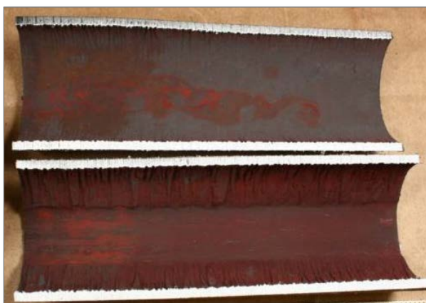
Corrosion and failure on the lower surface of a horizontal line etched due to low pH when steam condensed
