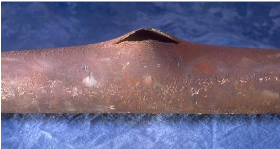
Thick lip failure due to metal creep from long term overheating Lines of stretch marks visible beside tube failure
