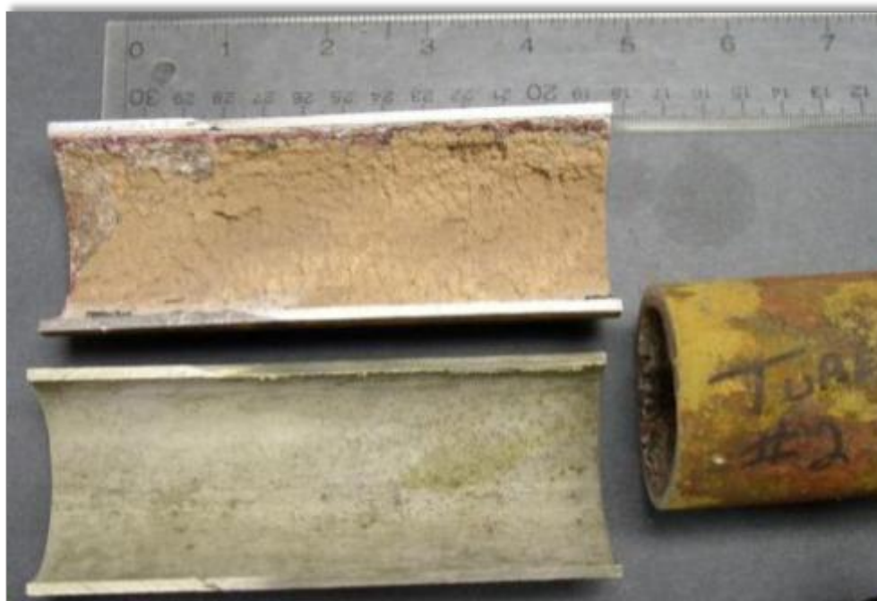
Tube with as-received (top) and as-cleaned (bottom) sections
