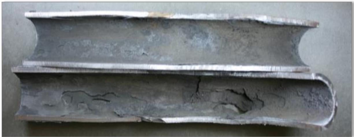
Superheater tube internal deposits
