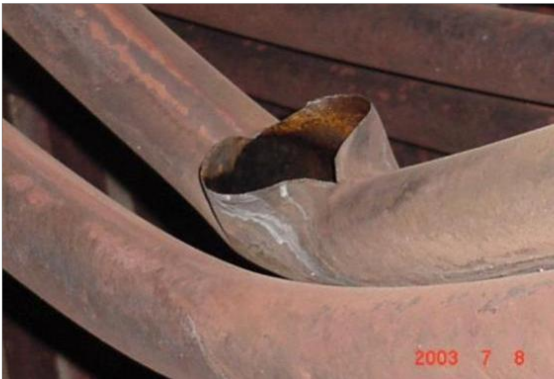
Thin lip failure due to rapid overheating
